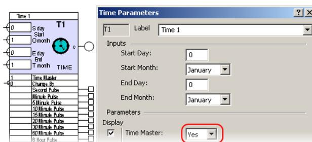
Once a time master has been configured, scheduled events can be configured within TREND 963 to synchronized the time master and hereby all controllers within its network with the system time.
